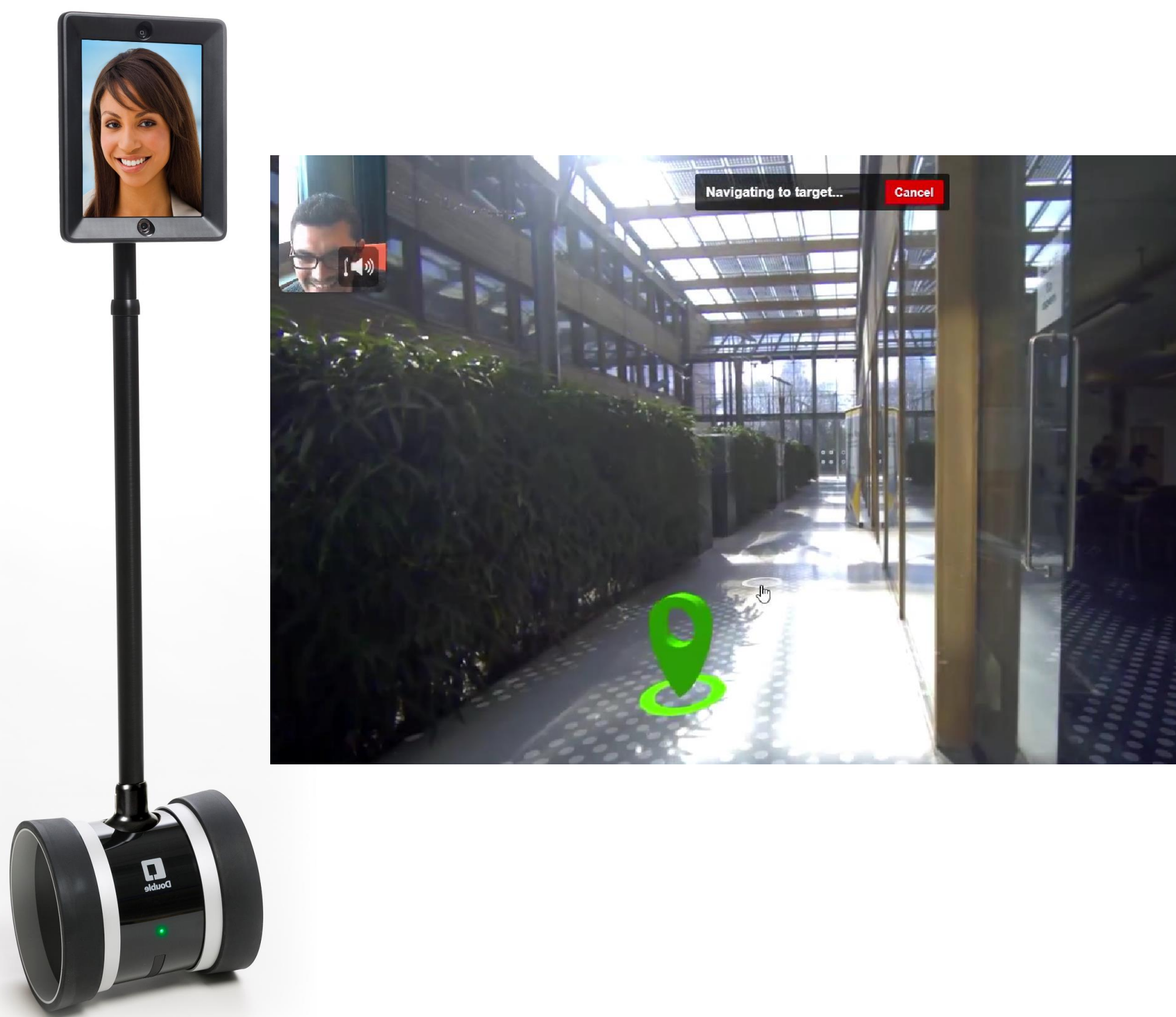
Figure 1: Left, The Double 2 Telepresence robot. Right, The point of view of a remote user, showing the interface of automated navigation on Double robots.
